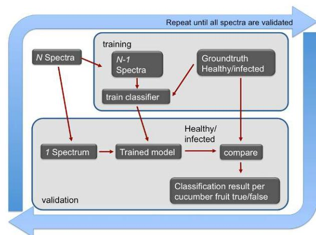
Fig. 8 Block diagram of the light transmission spectra based classification part using leave-one-out cross validation.
