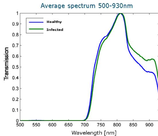
Fig. 7 Averaged light transmission spectra of all healthy and infected cucumbers in the dataset used in green and blue respectively. Wavelengths are presented on the x-axis and the responses of the spectrometer on the y-axis.
