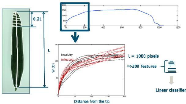
Fig. 4 Shape based classification method: cucumber widths extracted along the centreline (left) and the plot of a cucumber widths vs the distance from the cucumber tip (right). Each of the 200 widths represents a feature that is used by a linear classifier for the shape based cucumber classification.
