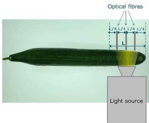
Fig. 6 Light transmission measurement near the cucumber tip:  $L \sim 0.2 \cdot \text{Cucumber length}$ .
